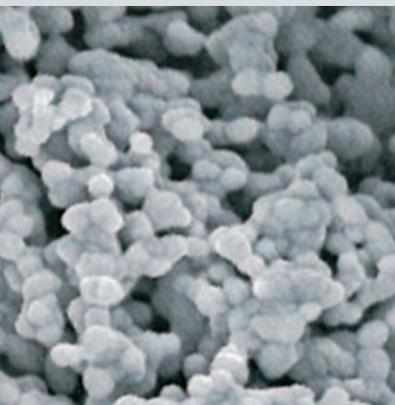
AgProtect™: Typical structure of a metal powder produced via inert gas condensation (nano powder). This antimicrobial nano silver (Ag) coating reduces pathogens on the microscope and their transfer to the users.
